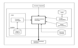
Figure 1. Proposed control access system architecture and operation
