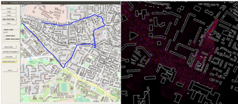
Figure 1. Simulation of a siren alert along an emergency vehicle path. The left figure is part of a city map, with a trip path used by many health transport vehicles having sirens. The right part displays a sample of sound pressure estimation in part of this path. Red pixels represent expected sound in streets.
