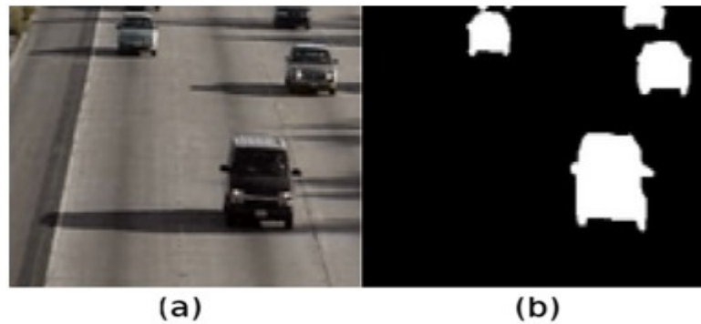
Figure 5. (a) Original color image. (b) Segmented image using Genetic Programming and algorithm proposed by (Perlin & Lopes, 2013).
