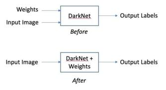
Figure 6. Visualization of the Model Change Before and After Static Compilation of Weights
