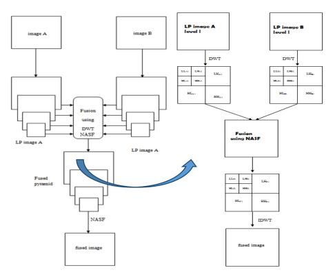
Figure 2. The proposed method Figure 3. DWT image fusion
