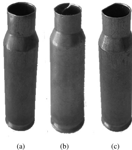
Figure 2. (a) Normal mouth, (b) mouth with split defect, (c) mouth with dent defect
