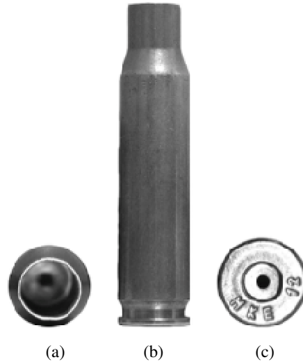
Figure 1. Parts of military cartridge case: (a) mouth, (b) cylindrical surface, (c) primer.
