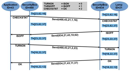
Figure 7. Simple Synchronous Method Example
