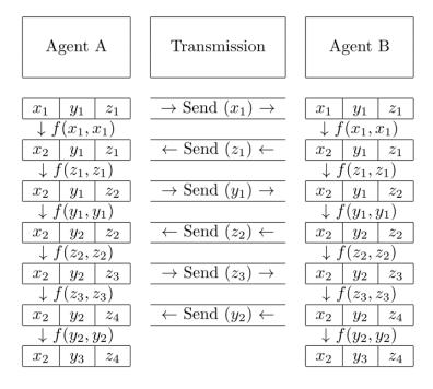
Figure 2. Simple Synchronous Method
