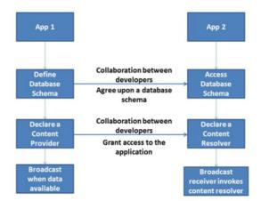
Fig. 3. Inter App interaction for Android platforms.
