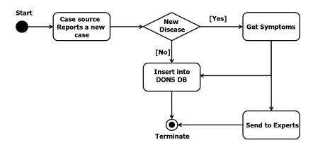
Figure 4: The ETL module activity diagram
