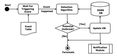
Figure 5: The Detection module activity diagram
