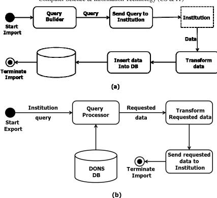
Figure 6: (a) The Import module (b) the Export module
