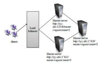
Figure 4. Master web servers based on cluster architecture
