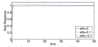
Fig 11. Step responses with ABS applied on motor 4
