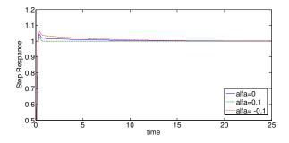
Fig 13. Step responses with FNN applied on motor 1
