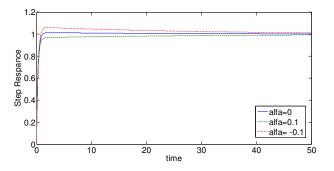
Fig 7. Step responses with SFL applied on motor 5
