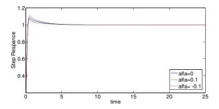
Fig 17. Step responses with FNN applied on motor 5
