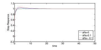
Fig 12. Step responses with ABS applied on motor 5
