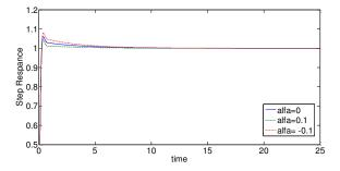
Fig 15. Step responses with FNN applied on motor 3
