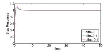
Fig 6. Step responses with SFL applied on motor 4
