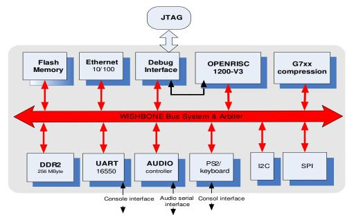
Figure 4 The VOIP Gateway general architecture
