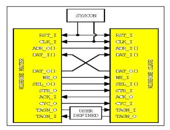
Figure 6. WISHBONE interconnect schema
