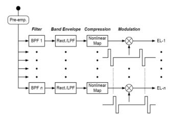
Figure 7. Block Diagram of CIS Algorithm
