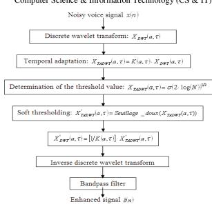
Figure 3. The block diagram of the proposed approach
