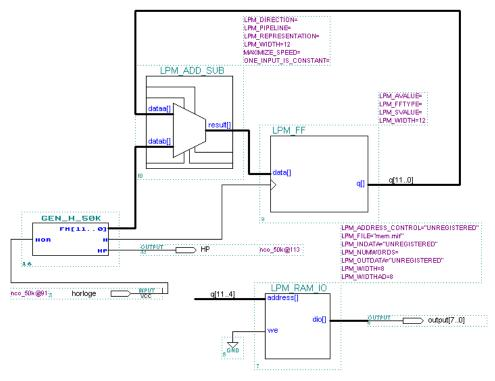
Figure 10. Complete diagram of BWT denoising in FPGA
