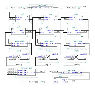
Figure 8. complete diagram of FIR filter in FPGA
