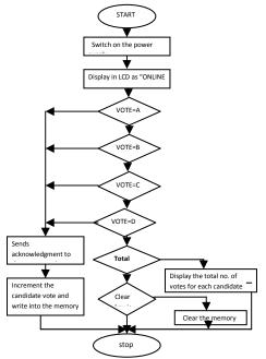
Fig. 3 Flow chart of Voting System using SMS
