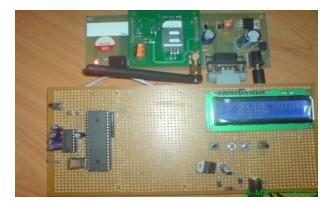
Fig. 3 Photograph shows Voting system using SMS
