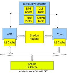
Figure 4 Architecture of Dual core with DPT
