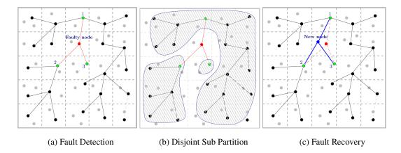
Figure 6. Fault Detection and Recovery
