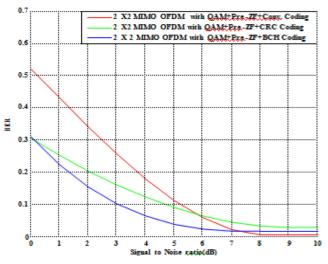
Figure 5 : BER Performance of a secured MIMO OFDM wireless communication with implementation of different Channel coding, Pre-ZF channel equalization and QAM digital modulation schemes.
