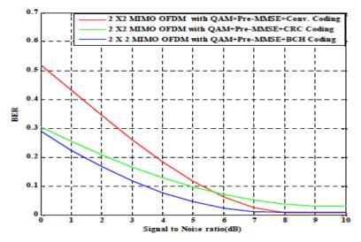
Figure 3 : BER Performance of a secured MIMO OFDM wireless communication with implementation of different Channel coding, Pre-MMSE channel equalization and QAM digital modulation schemes.
