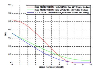
Figure 4 : BER Performance of a secured MIMO OFDM wireless communication with implementation of different Channel coding, Pre-ZF channel equalization and QPSK digital modulation schemes.
