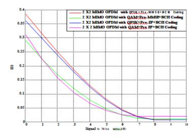
Figure 6 : BER Performance Comparison of the MIMO OFDM wireless communication system for different Pre channel equalization and digital modulation schemes under BCH channel coding scheme.
