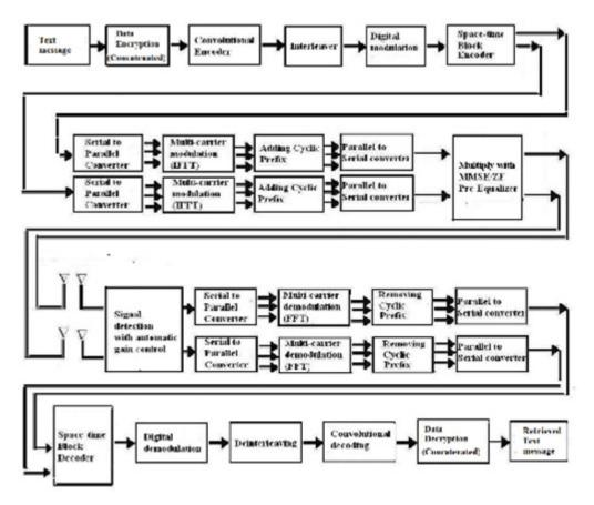
Figure 1: Block diagram of a Pre-Channel Equalization based secured MIMO OFDM wireless communication system
