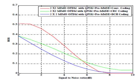
Figure 2 : BER Performance of a secured MIMO OFDM wireless communication with implementation of different Channel coding, Pre-MMSE channel equalization and QPSK digital modulation schemes.
