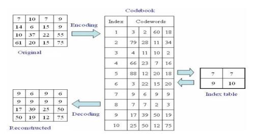
FIGURE 1. An Example of Encoding and Decoding by VQ
