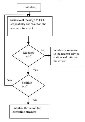
Figure 2. Work flow diagram of Health Monitoring system
