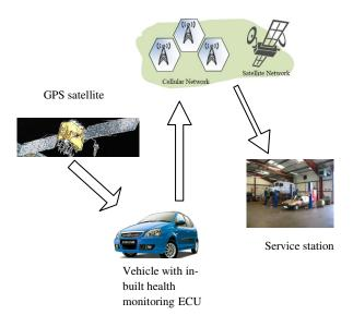
Figure 4. Deployment of Health monitoring ECU
