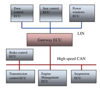
Figure 1. Schematic of the current In-Vehicle Network.
