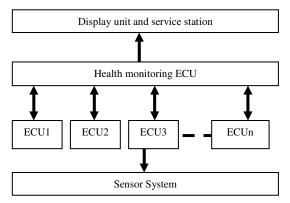
Figure 3. Block Diagram Of Health Monitoring System
