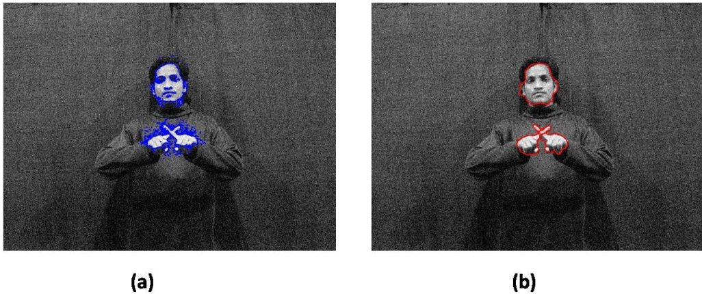
Figure 4. Example showing robustness of segmentation to noise. (a) is CV model and (b) Proposed method both with white Gaussian noise of \sigma = 2 and \mu = 0
