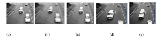
Figure 2: Filtering noise from an image. (a) Original image, (b) Noisy image, (c) Wiener filtered image, (d) Median filtered Image (e) 2D Filter Image
