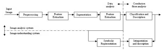
Figure 4: Block diagram for Feature Extraction Process
