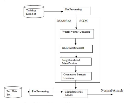
Figure 1: Proposed Framework for Anomaly Detection
