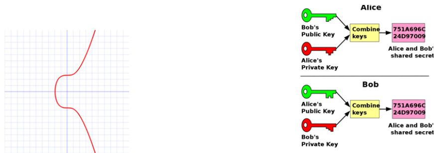
(a) Graph of secp256k1's elliptic curve (b) Simplified process of the Elliptic Curve y^2 = x^3 + 7 Diffie-Hellman (ECDH) key exchange
