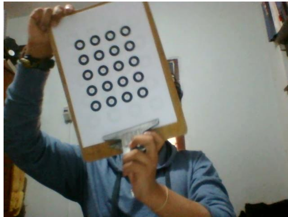
(a) Calibration pattern located at approximately half a meter of distance from the camera.
