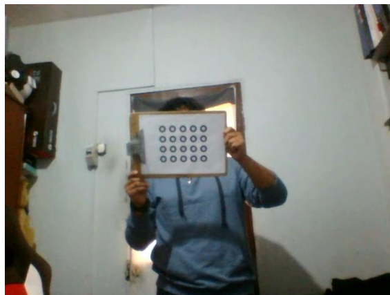
(c) Calibration pattern located at approximately a meter and a half of distance from the camera.
