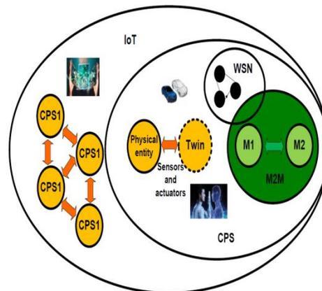
Figure 5. Synthesis diagram of IoT subsets
