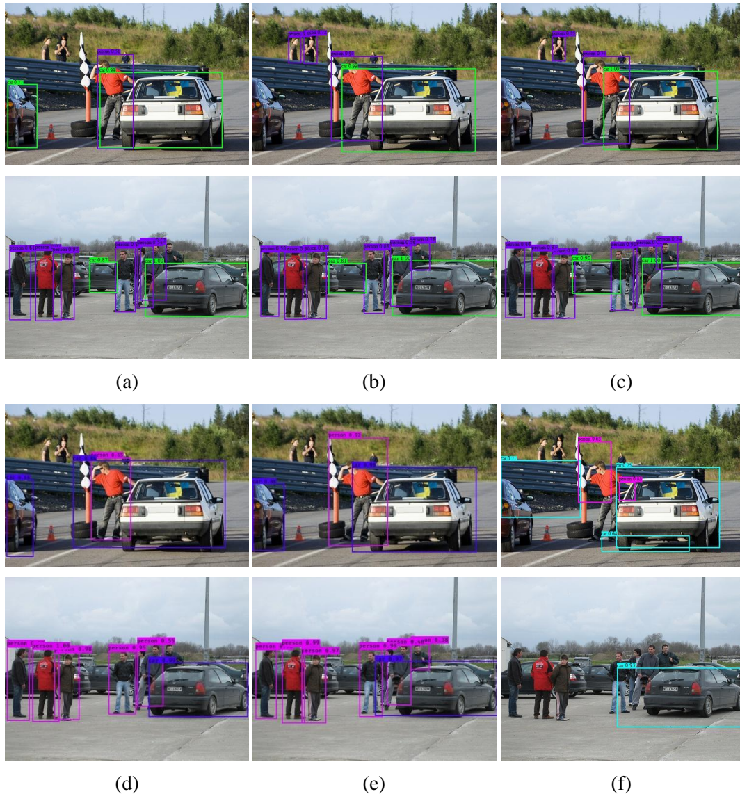
Figure 2. Object detection results: (a) SSD-MobileNetV2 (b) SSD-VGG16 (c) SSD-ResNeXt50 (d) YOLO-MobileNetV1 (e) YOLO-ResNet50 (f) SVM-HOG
