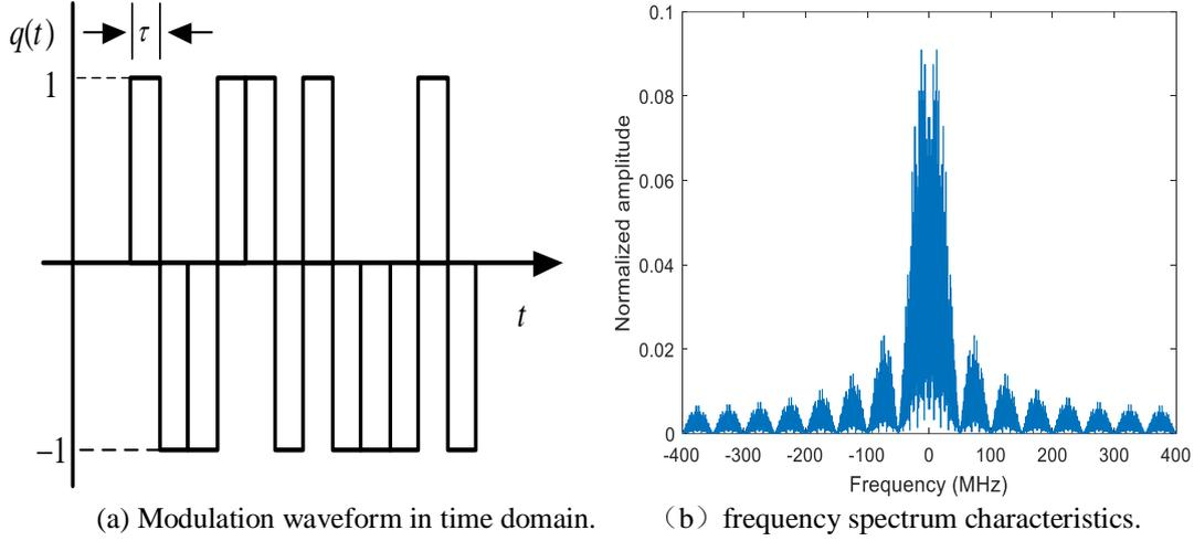
Fig. 3. The random code modulation waveform of the PSS.
