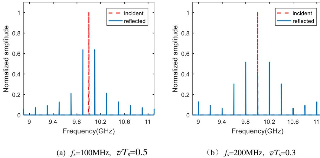
Fig. 4. The frequency spectrum of single frequency signal based on PSS modulation.
