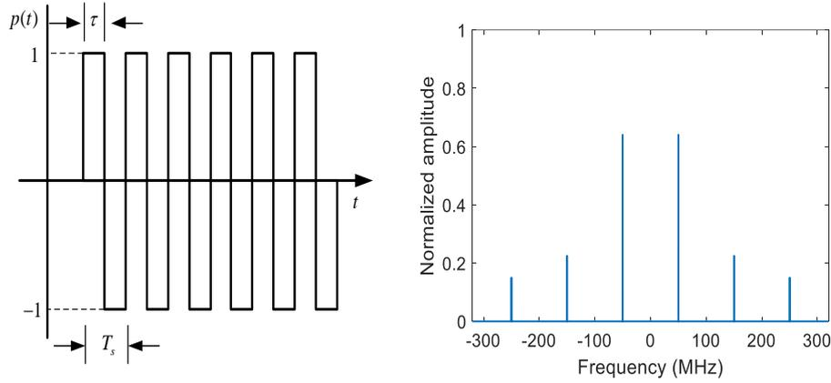
(a) Modulation waveform in time domain. (b) frequency spectrum characteristics.
