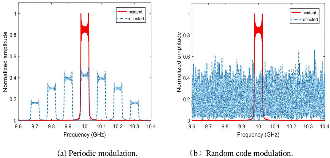
Fig. 5. The frequency spectrum of LFM signal based on PSS modulation.
