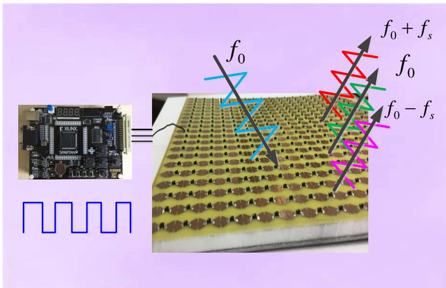
Fig. 6. Control device to PSS modulation diagram.
