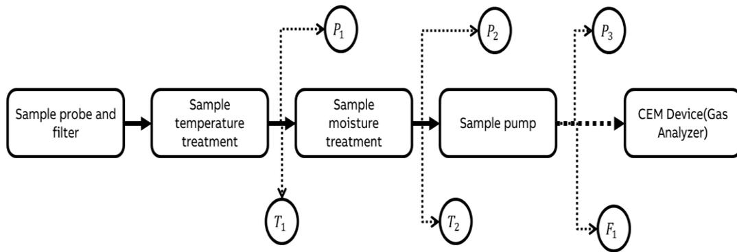
Figure 1: Block Diagram of Sample Handling System
