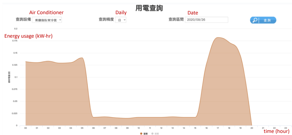
Figure 2: A visual example of energy consumption of the air conditioner in HEMS data.
