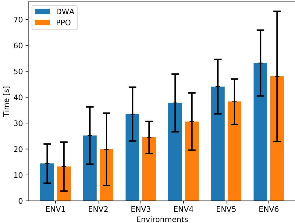
Figure 6: Average completion time for the DWA and our learned policy. The box height shows the average completion time and the whiskers illustrate the standard deviation. As can be seen, our trained policy outperforms the DWA in each environment. The difference is statistically significant in Env3, Env4, and Env5 according to a *paired* t-test at the 0.05 level.
