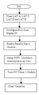
Figure 7. The Flow Chart of the Initialization Sub Routine Interrupt
