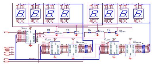
Figure 4. Circuit Diagram of LED Display Module
