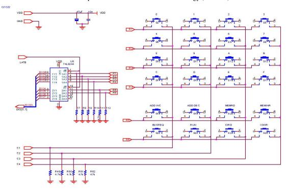
Figure 3. Circuit Diagram of Keypad Module
