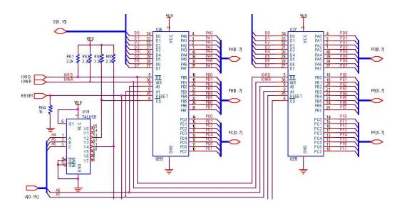
Figure 5. Circuit diagram of I/O port
