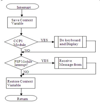
Figure 8. The Flow Chart of the Interrupt Subroutine
