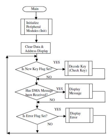
Figure 6. The Flow Chart of the Main Routine
