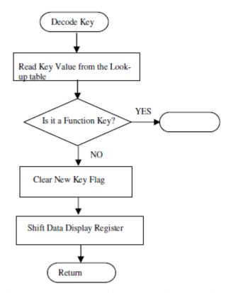
Figure 9. The Flow Chart of the Key Decoding Subroutine
