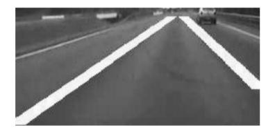
Fig.9. LBROIs corresponding to initial lane segmentation using the linear model.
