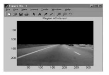
Fig. 3. Road surface as the object/region of interest. Other objects/background are converted to black (0).
