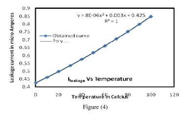
The above given plot is the variation of leakage current with temperature. The ideal behavior of leakage current with temperature is super linear curve. The result obtained from our simulation follows the ideal curve. Temperature is varied from 0° C to 100°C by keeping  $V_{dd}$  constant and  $I_{leakage}$  is calculated. The figure 5 shows the variation of leakage current versus supply voltage.
