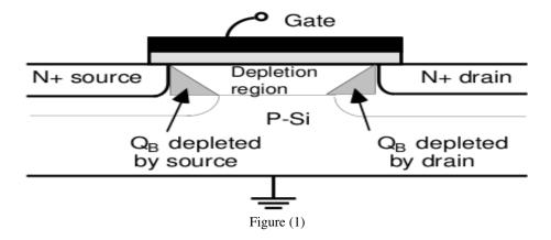
If the channel length becomes too short, the depletion region from the drain can reach the source side and reduces the barrier for electron injection. This is known as punch through.
