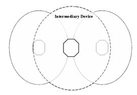
Figure 3.Expanding range using intermediate device
